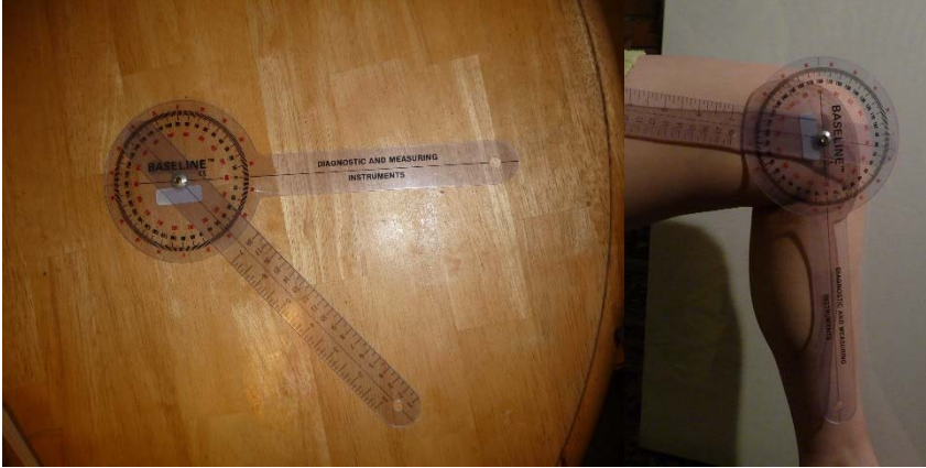
Figure 1. The protractor (Baseline™ Instruments, Country Technology, Inc, P.O.Box 87, Gays Mills, WI 54631-0087) is our primary tool for measuring the minimum angle (maximum bend) of subjects' knees.
